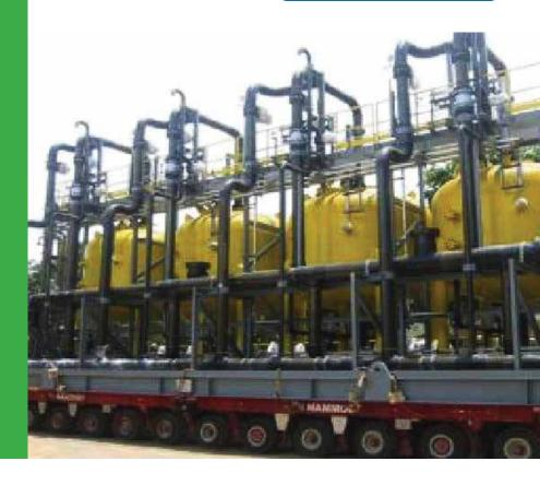
We provide complete produced water treatment solutions for both offshore and onshore applications. For onshore applications, our solution typically comprises corrugated plate separation (CPI), induced gas flotation (IGF), dissolved gas flotation (DGF) and multimedia filtration for polishing. For offshore applications, our solution typically comprises of deoiling hydrocyclones and Compact Flotation Unit (CFU).
