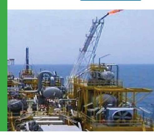
We offer various solutions for hydrocarbon dewpointing depending on the allowable pressure drop, degree of dew point suppression required, plot space limitations, etc. HC dew points can be achieved by applying either the Joule-Thompson valve-based processes or a chiller with refrigeration packages or turbo expander for high-performance recovery.
